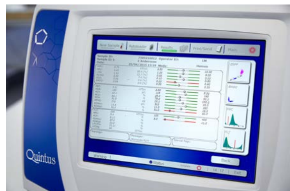
Fig 2. The large touchscreen of the Quintus analyzer provides plenty of room to display all 26-parameter results together with scattergrams, histograms, and system messages.
