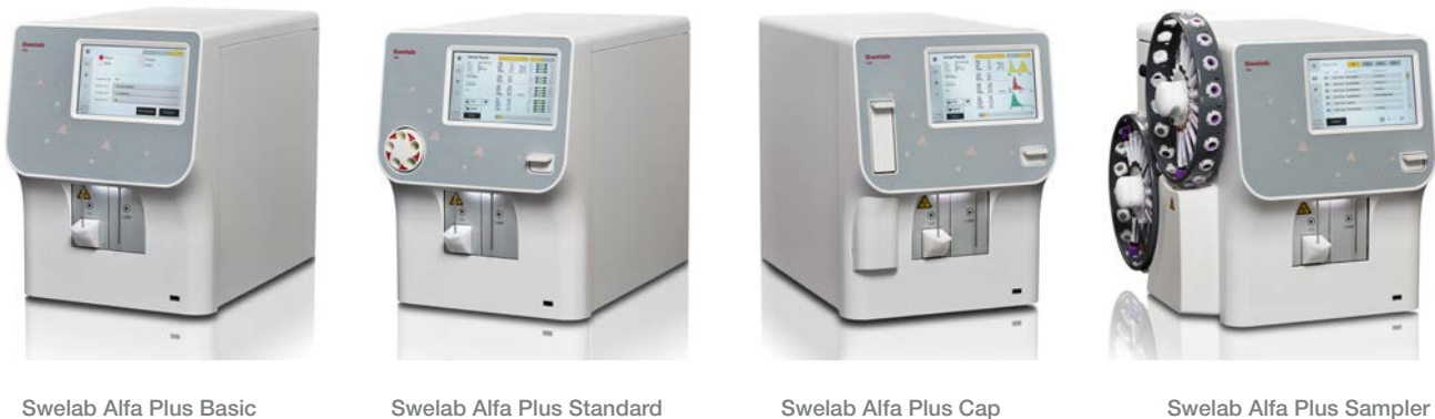
Figure 1. Swelab Alfa Plus automated 3-part hematology analyzer is available in four versions. While both Basic and Standard support open tube aspiration, Standard features an integrated mixer. Cap and Sampler support closed-tube aspiration to minimize the risks associated with contaminated blood. In addition, Sampler is equipped with an Auto Sampler for up to 2 × 20 samples - just load and walk away.
